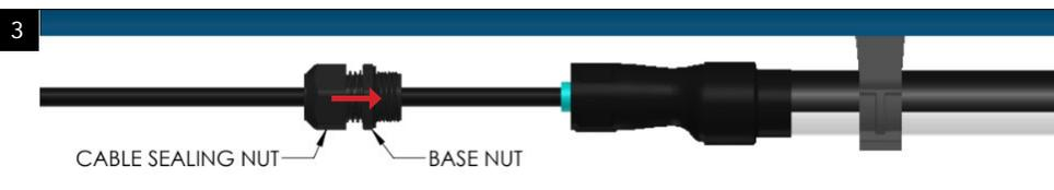
Thread the cord-grip onto the input end of the fixture. First, tighten the base nut. Then tighten the cable sealing nut. (40-45 in-lbs is recommended.)
